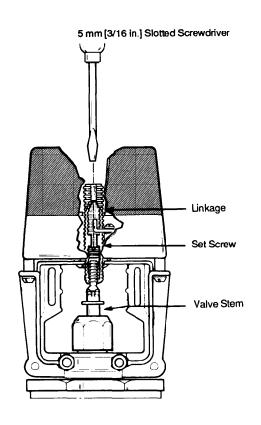
FIG. 6. -- LOCKING ML7984 DRIVE SHAFT TO VALVE STEM
